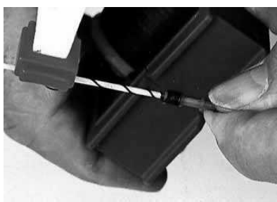
At the outer shoulder, the thread will return to the string through the free, out-going thread indentation.
