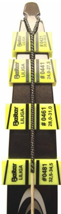
The Beiter Limb Tip Line Gauge helps to determine limb straightness and torsion. One set of 4 gauges (#0421/0441/0461/0481) has sizes from 20,0-34,5mm: at least three of them can be placed on the tips of each available limb on the market.
